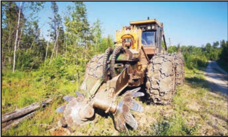
This big machine is a hydraulic power trencher. Its large discs rotate, and down pressure is applied to expose mineral soil in trenches. The trenches are one to two feet wide and spaced six feet apart. (Supplied photo)
