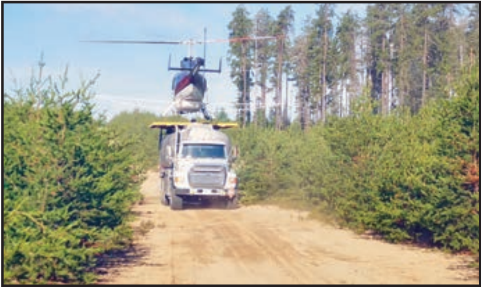
This helicopter is used for aerial herbicide application. It is pictured here landing on a mix rig used for both refuelling the helicopter and for refilling a tank containing a mixture of herbicide and water. (Supplied photo)
